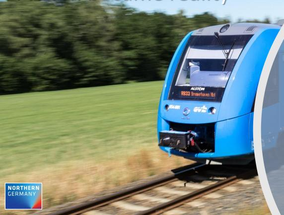
ALSTOM from Salzgitter has developed the world's first passenger train powered by a hydrogen fuel cell. Its top speed is 140 km/h, and it can cover up to 1,000 km. This CO<sub>2</sub> emission-free train is low-noise and emits only water vapour and condensation.
